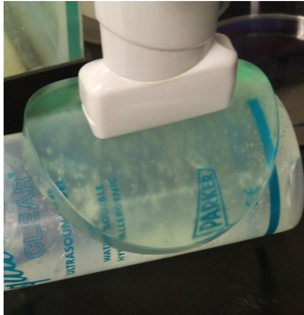
Figure 2.11: Bubble imaging test using the conforming gel pad
