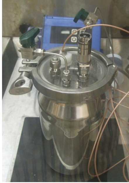
Figure 2.5: Angled transducer design ready for mercury experiment inside fume hood.
